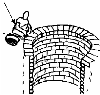
Figure 3: dressing the top of the pit
